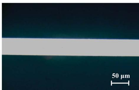
**Fig. 4** Optical image of a channel fabricated by  $\mu\text{CECE}$  (the opaque parts are the metal mask and the transparent ones are the glass substrate).
