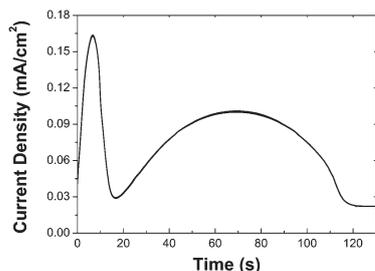
**Fig. 3** Chronoamperometry curve of Au/Cr/glass in 0.2 mol L<sup>-1</sup> KCl solution at 1.0 V vs. SCE.
