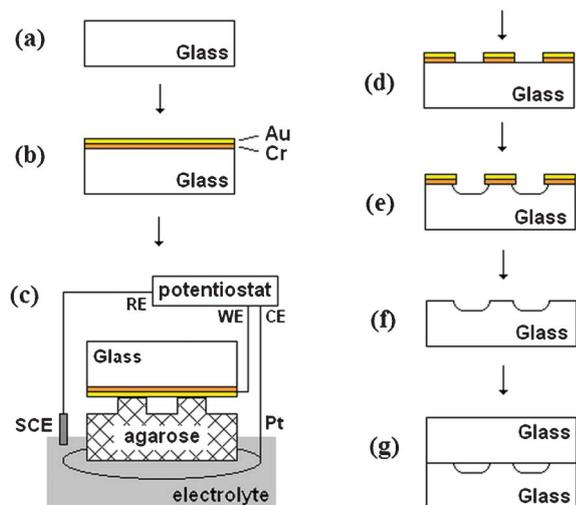
**Fig. 1** Schematic illustration of the process for fabrication of a glass based microchip: (a) bare glass; (b) glass coated with Cr and Au layer; (c)  $\mu$ CECE; (d) exposed metal mask etched; (e) exposed glass etched; (f) metal stripped; (g) glass cover plate bonded to form microchips.
