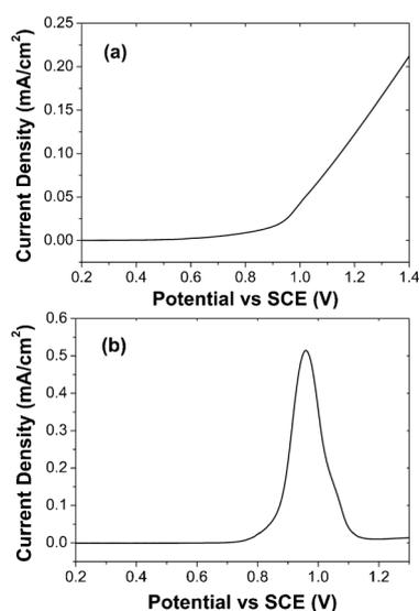
**Fig. 2** Cyclic voltammogram for (a) Cr and (b) Au film deposited on glass in a solution containing 0.2 mol L<sup>-1</sup> KCl (scan rate: 50 mV s<sup>-1</sup>).
